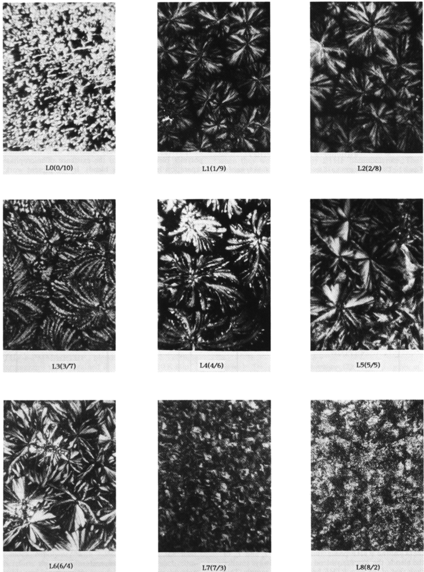
Figure 6 Optical micrographs of the L series of compatible PTHF- b -PMMA/PTHF blends cast from chloroform and isothermally crystallized at 288 K (magnification 910 \times )
